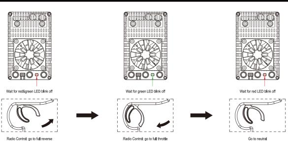
1. ESC power off- go to full reverse-ESC power on--wait for red/green LED blink off
