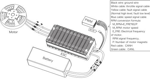
Yellow cable: fault signal cable (Normal high level, fault low level) P: Number of motor magnets
